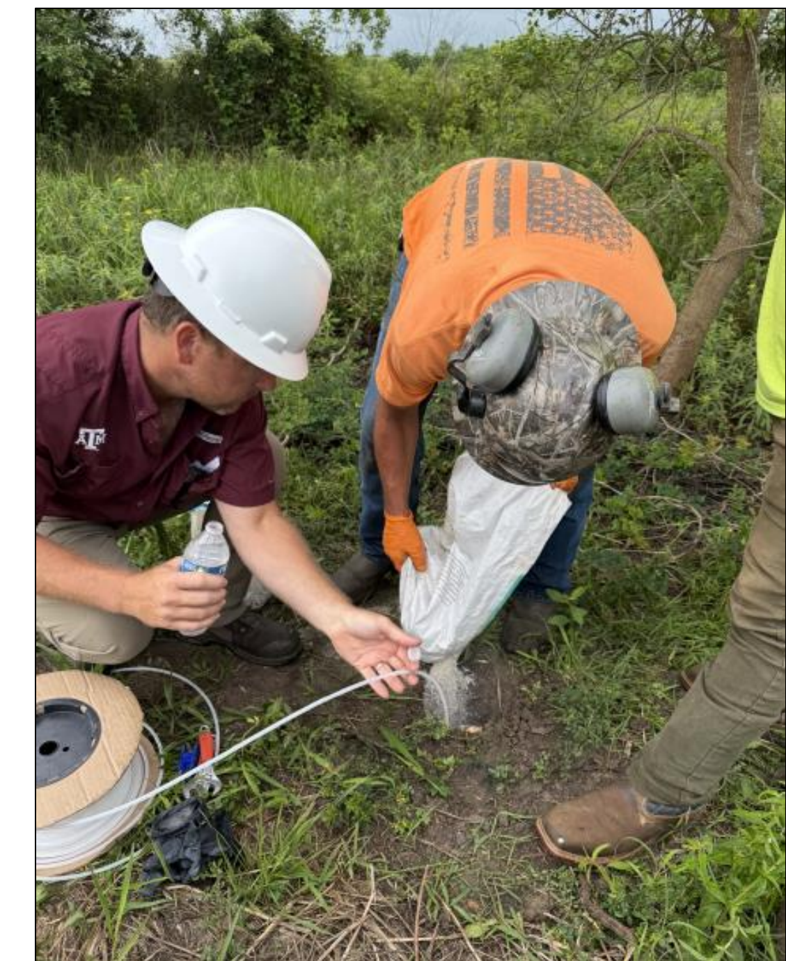
Soil Gas Probes Installation (Summer 2025)
